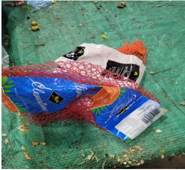
Figure 3.19 Contamination - Plastic Laminates
