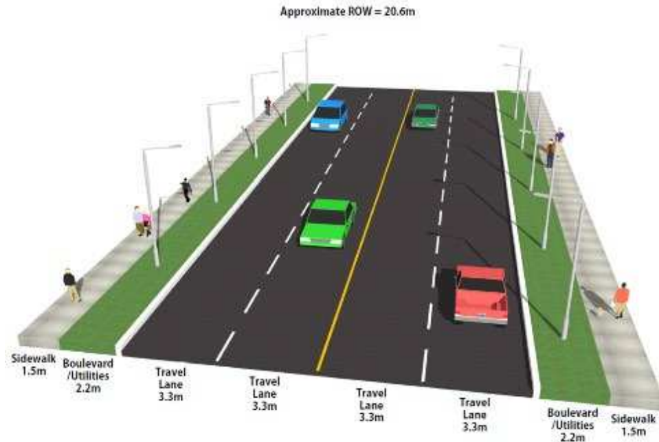
Figure 3-20: Existing Cross Section for North Front Street
