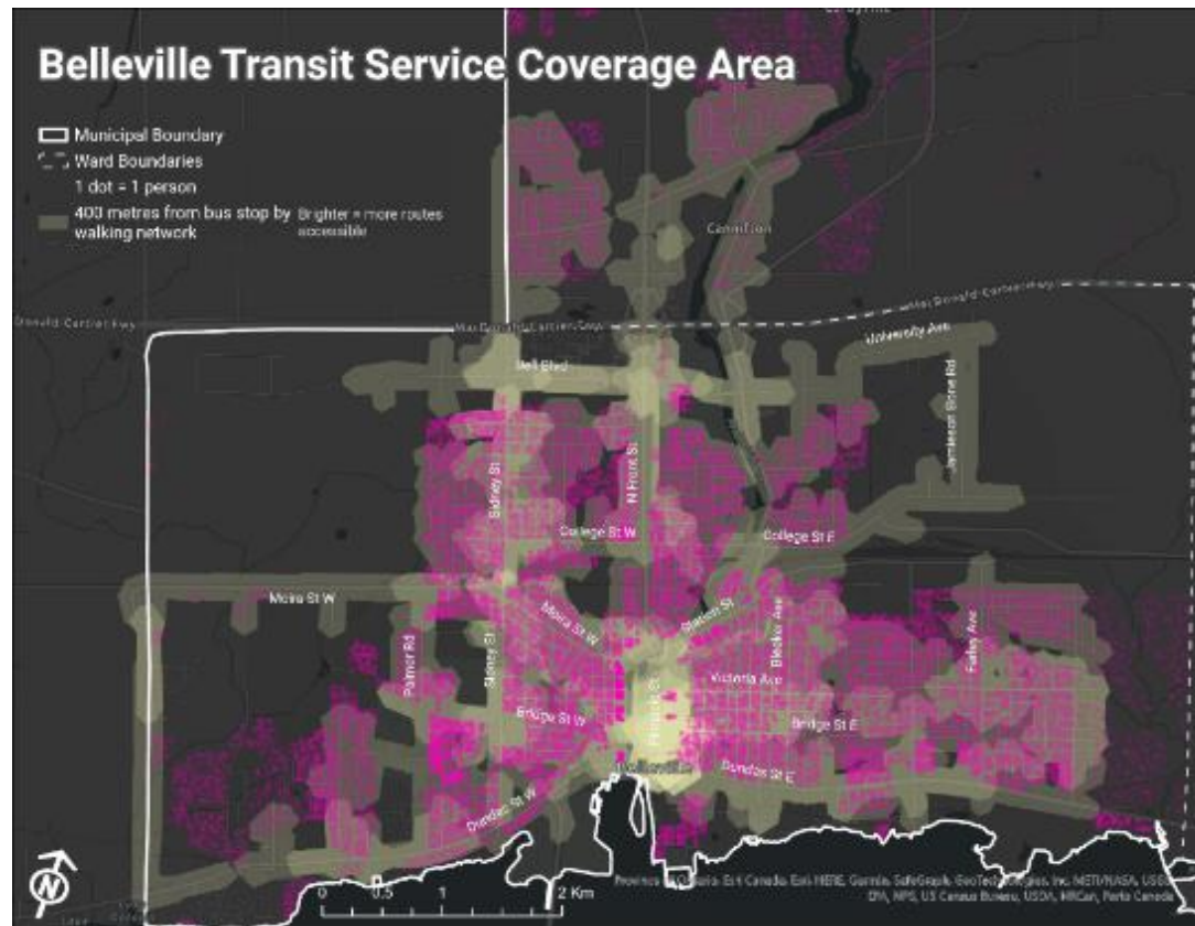
Figure 23: Existing bus network coverage area assuming a 400-metre walk along the road network to access a bus stop, where brighter yellow indicates more bus services available
