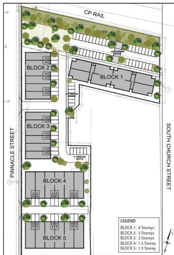
Figure 2: Site Concept Plan for 105 Pinnacle Street (not to scale; image source: Hobin Architecture Incorporated)
